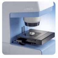
The LUMOS provides plenty of space for the sample and a large working distance.
