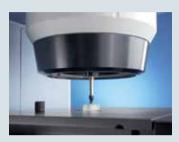
The LUMOS includes an 8x objective which is used in transmission, reflection and ATR mode. In transmission and reflection the ATR crystal is inserted into the objective. For data acquisition in ATR the crystal is positioned into the IR focus by an encoded piezo drive. An integrated pressure control ensures the constancy of the pressure applied from the crystal to the sample which is essential for mapping and imaging experiments.
