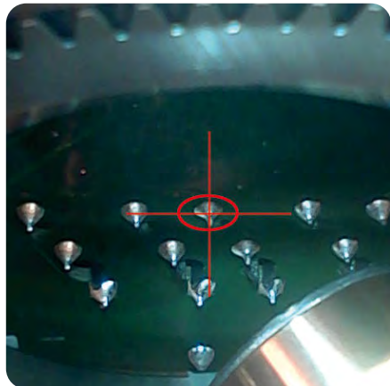
Sample positioning with video camera
