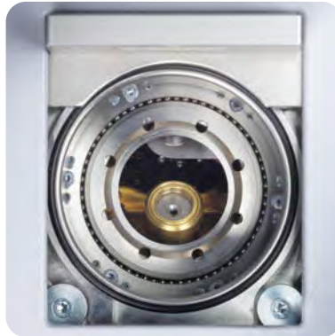
Sample rotation for accurate results
