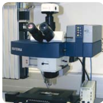
The SENTERRA can be mounted on a z-stage that allows access to large samples.
