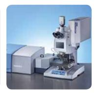
To analyze samples with highest lateral resolution, the TENSOR II can be extended by FT-IR microscopy and FT-IR imaging.
