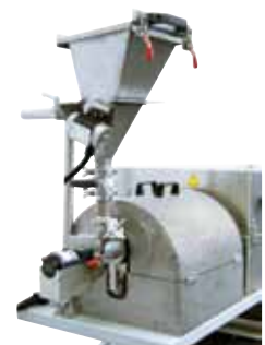
Vibration generator at the charging funnel for improved powder supply
