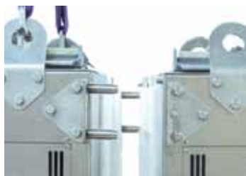
Bolts for connection of two separated half furnaces
