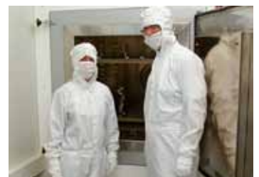
Industrial oven N 250/65 HAC with particle-free oven chamber. For charging, furnace door is located in cleanroom, class 100, furnace chamber in greyroom behind.
