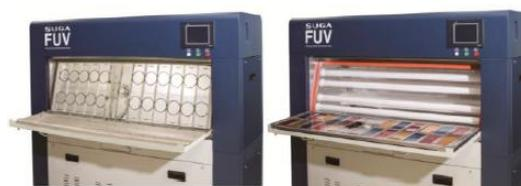
The Quick View System™ fixes the specimens to the chamber door, allowing for the viewing of the condition of all the specimens in a single motion.
