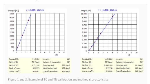
Within the method up to three calibration ranges can be linked to each parameter in order to cover an over-all working range of up to three magnitudes. With the NPOC/TN $_{\rm b}$  method three NPOC and two TN $_{\rm b}$  multi-point calibration ranges were linked as follows:
