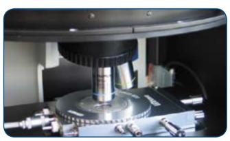
Heating/cooling stage used in the SENTERRA II.
