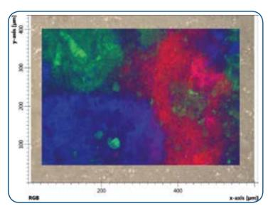
High resolution Raman image of a painkiller tablet showing the distribution of 3 different API's on top of the visual microscopic image.
