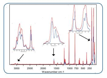
SENTERRA II provides the full spectral range even at high resolution. Spectra of triptycene measured at a resolution of  $4 \text{ cm}^{-1}$  (red) and 1.5 cm<sup>-1</sup> (blue).
