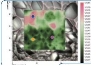
The permanent wavenumber calibration of SENTERRA II allows the determination of crystallinity dependent variations on a silicon surface with the highest precision. The spectra colors match the selected measurement positions on the Raman image.
