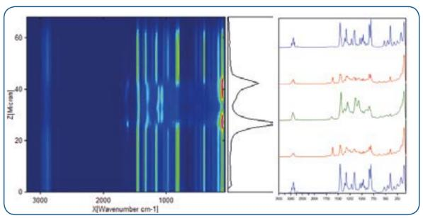
Raman depth profile of a 5 layer polymer laminate revealing intermediate layers with diameters less than 3µm and 4µm.
