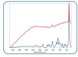
Spectra of caolinite showing the effectiveness of various laser excitation lines. Red: 785nm, blue: 1064nm
