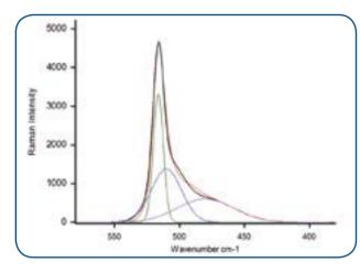
Characterization of the crystallinity of a silicon thin film on a solar cell. The spectrum (red) was measured with very low power to avoid any sample damage.
