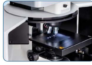
Validation plate with integrated standard materials for automated instrument qualification tests
