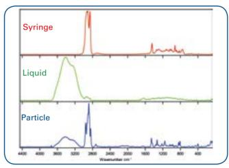
Failure analysis in a pharmaceutical product: Non-invasive analysis of a particle in a liquid filled syringe. Confocal measurement provides spectra of the syringe (red), liquid (green) and particle (blue).
