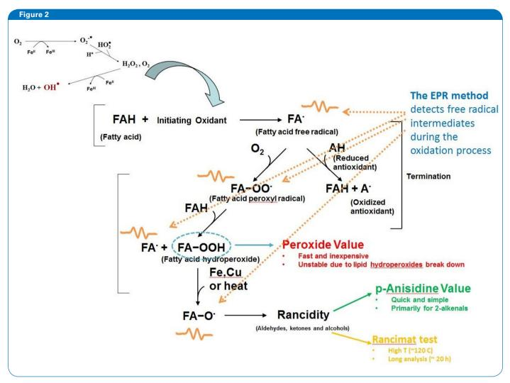
Free radical oxidation and typical test methods.
