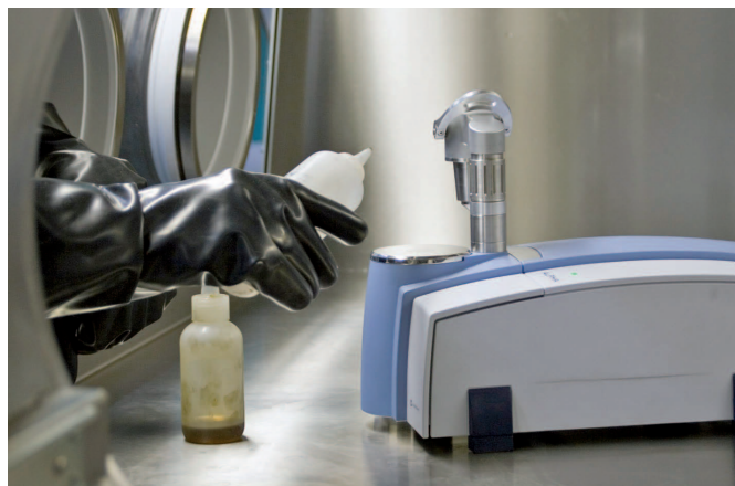
Figure 6: ALPHA spectrometer inside a glovebox.
