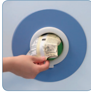
TD-NMR can inspect even through the packaging material of diverse samples, like for quick fat content determination.
