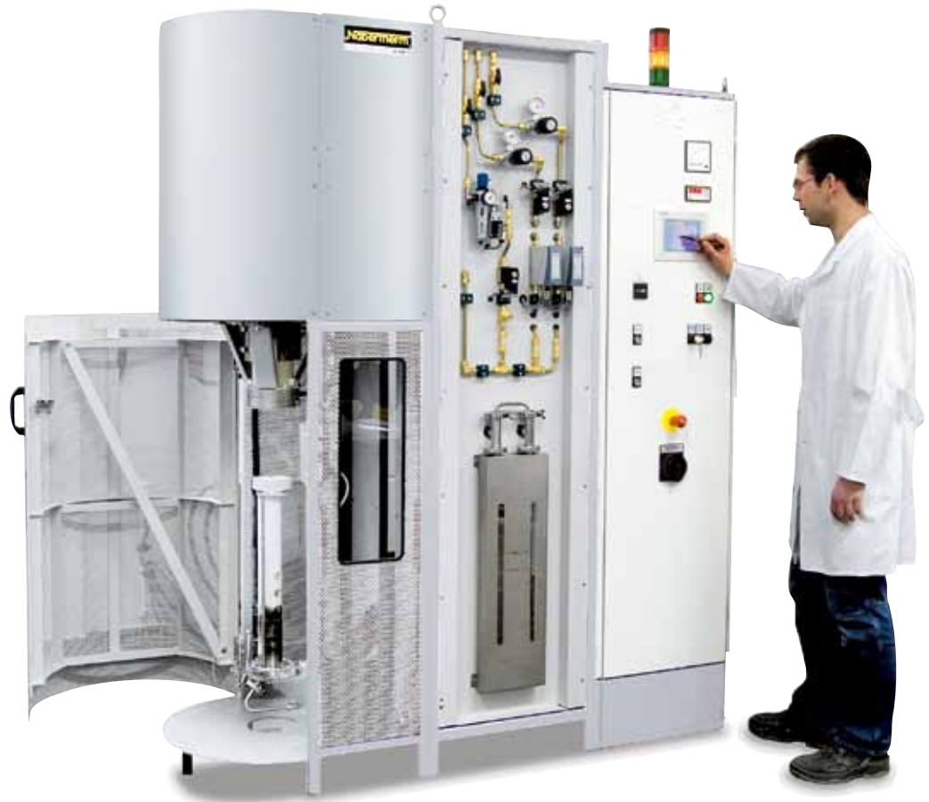
RHTV 120/480/16 LB in customer-specific design with working tube closed at one side, protective gas and vacuum option as well as with electric screw drive of the lift table
