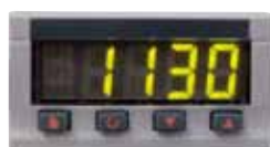
Over-temperature limit controller
