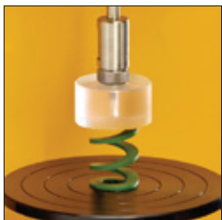
TA-11 Spring rate test measures force vs distance of springs
