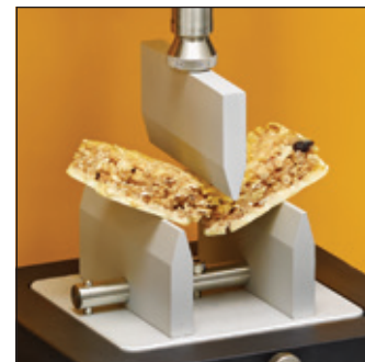
TA-TPB F Three Point Bend Fixture is used with TA7 blade from general probe kit. Rotary Base Table required. Small scale version TA-JTPB is available.
