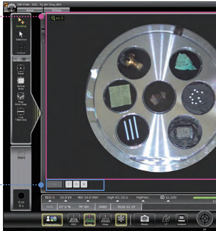
Display of elemental composition and "Alert" on live image
