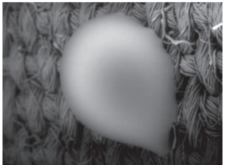
Specimen : Water droplet on a water-repellent textile. Accelerating voltage : 30 kV Magnification : × 80 Low-vacuum mode : 650 Pa Backscattered electron composition image.
