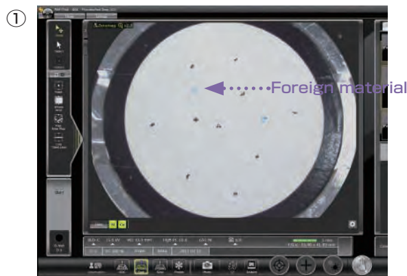
① Acquire a CCD image*1 of the filter mounted on a 3-inch holder.
