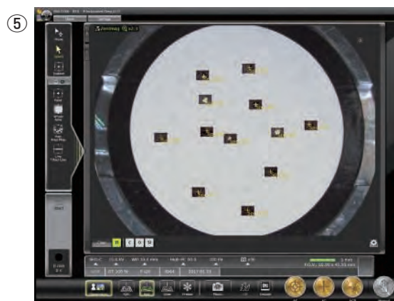
Repeat steps ① to ④ to set positions for analysis of all the foreign materials . When you click the Start button, automated multiple-area serial analysis is performed and the analysis results are stored.
