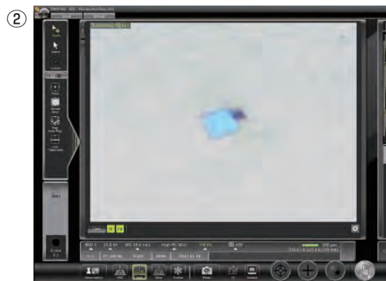
② Magnify the CCD image*1 using Zeromag to confirm a foreign material.
